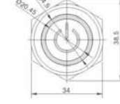
HBS1GQ30F-11ET 自锁式/40 H could be: Momentary type 34 Latching type 40
